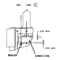
When replacing brushes or the armature, the dimensions shown must be as specified.
