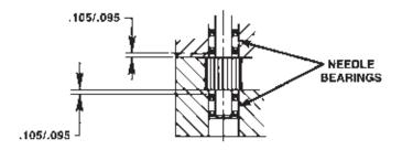
When replacing the needle bearings on the drive gear of the basic pump, the dimensions shown must be as specified.
