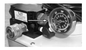
Figure 6. Pressure Gauge Installation
