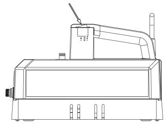
Figure 7. PE10 Motor Control Switch
