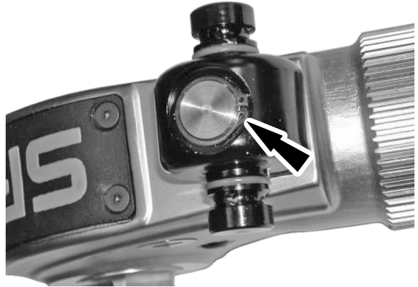
Figure 14. Swivel Banjo Circlip Removal
