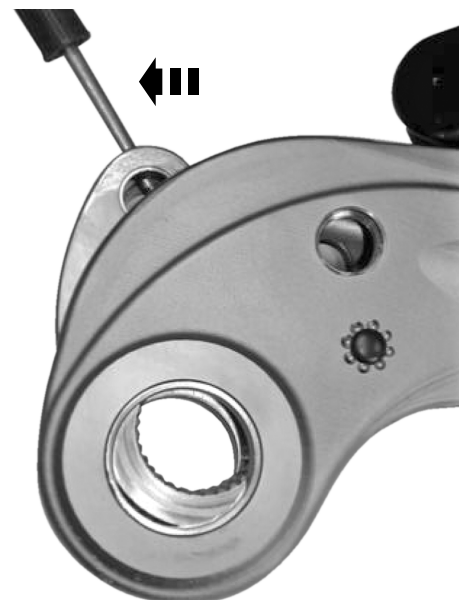
Figure 8. Drive Assembly Removal
