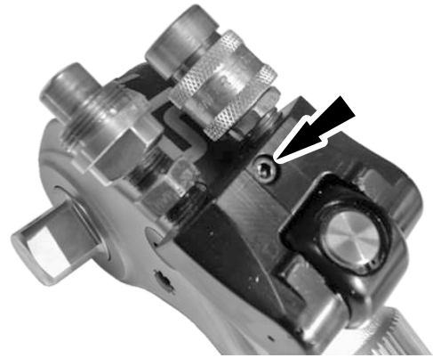
Figure 11. Swivel Yoke Screw Removal
