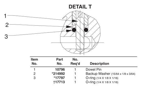
Part numbers marked with an asterisk (\*) are contained in Repair Kit No. 300651. Part numbers marked with a dagger (†) are contained in EPR Seal Kit No. 300653.
