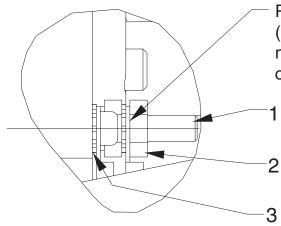
Power Cord Ground (Must be isolated between nuts and can be at top or bottom of stack.)
