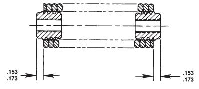
Spring must not extend beyond threads of spring retainer on either end. Stretch, clean and lubricate before assembly.
