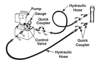
A double-acting cylinder or ram can be either extended or retracted hydraulically.
