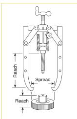
Remove gears, bearings, and other press-fitted parts with speed and ease.
